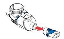
Step F4: Gently pull up on the tab to open the Handset and remove the Blue Valve (F-4).
