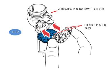
Squeeze the two flexible plastic tabs together while inserting the metal arms and flexible plastic tabs into the Medication Reservoir (**H-5c**). You should feel the flexible plastic tabs "grab" as you insert it.
